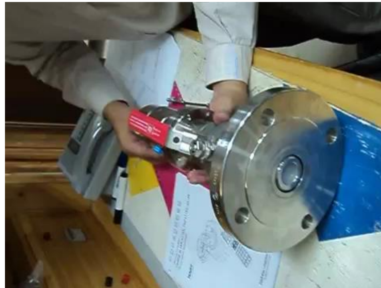
Overview of the retractable assembly
